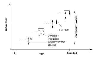
Figure 33. Combined FSK and LFM Waveform (N Corresponds to the Number of LFM Steps)
