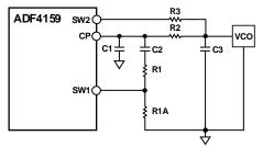
Figure 45 Fast-Lock Loop Filter Topology—Topology 1
