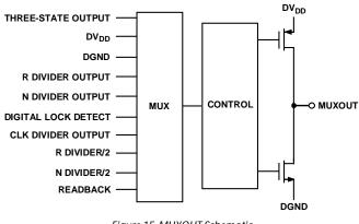
Figure 15. MUXOUT Schematic
