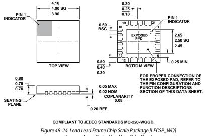
4 mm × 4 mm Body, Very Very Thin Quad (CP-24-7) Dimensions shown in millimeters
