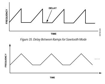
Figure 36 Delay between ramps for triangular mode
