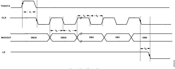
Figure 3. Read Timing Diagram
