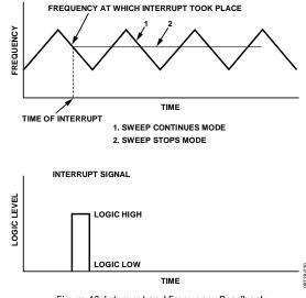
Figure 42. Interrupt and Frequency Readback
