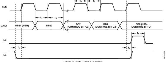
Figure 2. Write Timing Diagram
