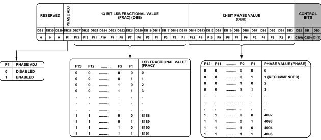
\*THE FRAC VALUE IS MADE UP OF THE 12-BIT MSB STORED IN REGISTER 0, AND THE 13-BIT LSB REGISTER STORED IN REGISTER 1. FRAC VALUE = 13-BIT LSB + 12-BIT MSB × 2<sup>13</sup>.
