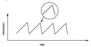
Figure 40 Fast Ramp Mode
