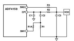
Figure 46. Fast-Lock Loop Filter Topology—Topology 2Spur Mechanisms
