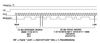
Figure 43 Reading Back Single Bits to Determine the Output Frequency at the Moment of Interrupt
