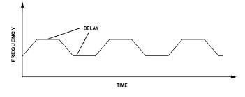
Figure 37 Delay between ramps for clipped triangular mode
