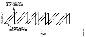
Figure 34. Delayed Start of Sawtooth Ramp
