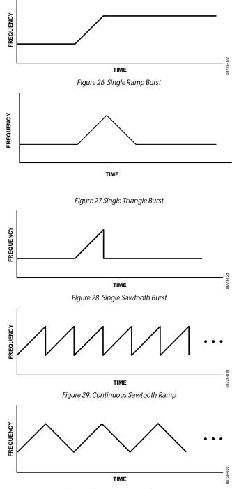
Figure 30. Continuous Triangular Ramp
